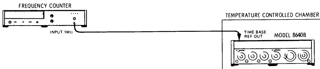
Figure 4-29. Internal Reference Accuracy Test Setup
